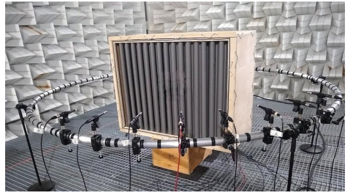
(a) Proxy buffet in anechoic chamber.
