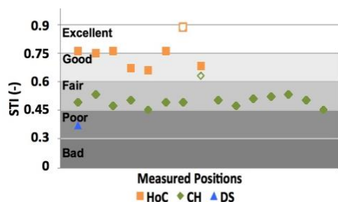
Figure 9 – STI results from the three spaces across the different measured positions
