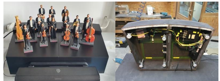
Figure 3 – left: the OrchestraBox with all musician markers, right: the underside of the box with the RFID antennas
