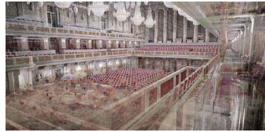
Figure 3 – Laser scan data during the digital survey of the Great Hall in the Konzerthaus Berlin
