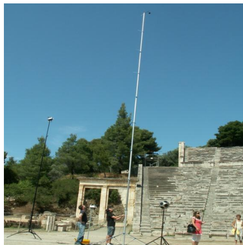
Photo 1- Orchestra Area: Dodecahedron, WS1, WS2, Orchestra Receiver 90° as fig.14a
