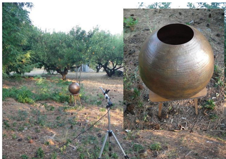
Figure 3. Photograph of the new test subject, a copper sphere of 40cm diameter with a 15.1cm opening and a thickness of 1.2mm
