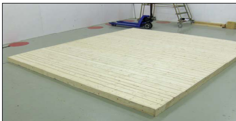
Figure 3 - Test elements on floor in reverberation room.
